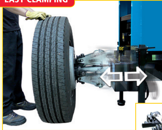
Hydraulic In-Out Movement
